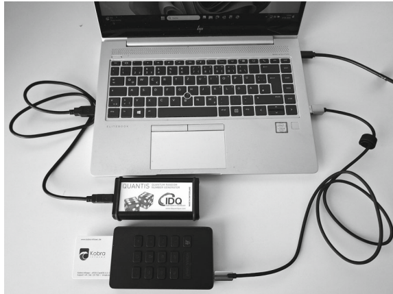
Fig. 5.3 Activation of a secure storage medium with PIN and smart card
